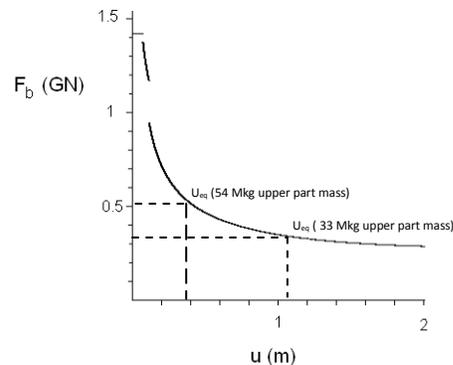
Fig. 1. Diagram of load vs. displacement during axial deformation and buckling
